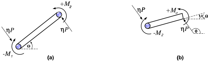
Figure 10. Free body diagrams of the pseudo rigid body model components: (a) the intermediate link with a length of (1 - \gamma_1 - \gamma_2)l , and (b) the output link with a length of \gamma_2 l .
